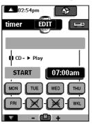
8. Scroll down to display the second timer control panel in which you can set the stop time.
